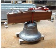
Photo courtesy of **John Taylor & Co.** From their website: "restoration work to be carried out on two swing chime bells that hang in a composite Aggett of Chagford bell frame. The bells will be lifted from their pits and their bearings cleaned. The existing fittings will be overhauled, and new rope bosses will be supplied and fitted. New bell ropes will be manufactured and fitted to complete the work."
